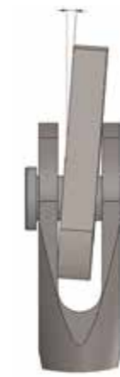
Additional misalignment with spherical bearing
